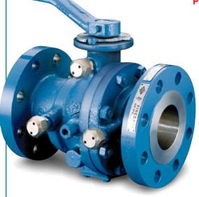
FA Ball Valves are well suited for sealing fluids, concurrently, at both ends. The bleed valve (21) provides a safe and convenient method for checking closed valve seat sealing effectiveness as required for Double Block and Bleed valves.
